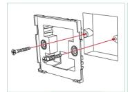
1. Remove the plastic frame and screw from the packaging box,and then install and fix the plastic frame to the 86 mounting box inside the wall after the wire is threaded out of the plastic frame.
